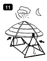
When not in use, swing the reflector dish upside down to protect it from rain.
