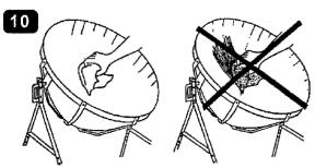
Use only soap and a soft cloth for cleaning the reflector. Cooking power will be lost by scratching the surface.
