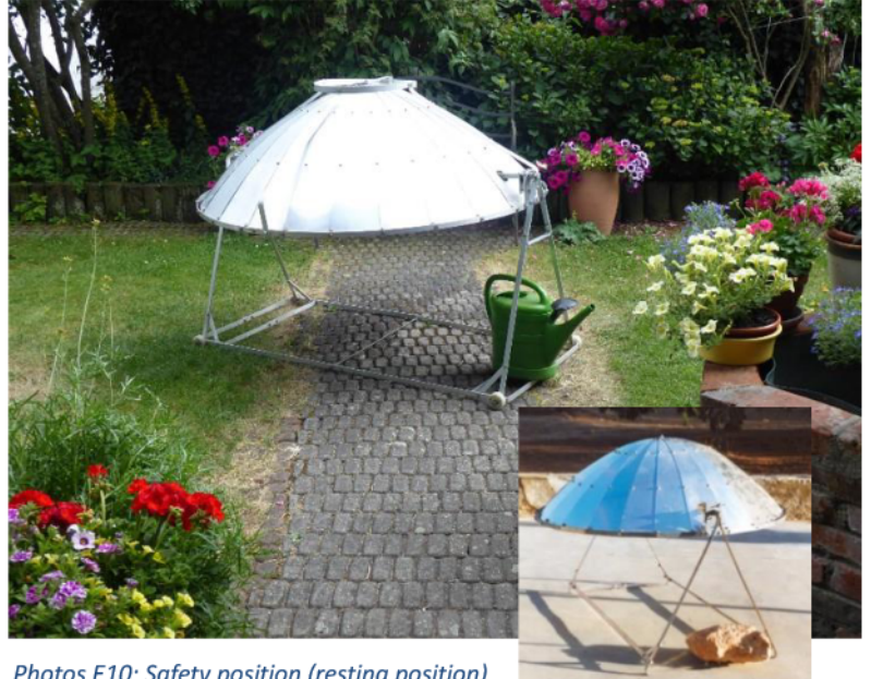
Photos E10: Safety position (resting position) when the solar cooker is not in use
