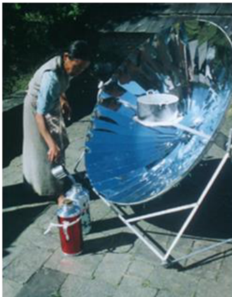
Photo A2: Thermos flasks in combination to the parabolic solar cooker (courtesy K. Schulte: SK14-Project Solar Cookers for Nepal, Rotary Sweden)
