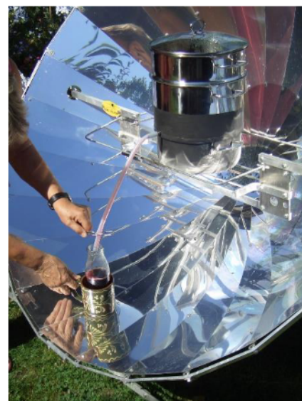
Photo E8: Steam juicer heated by the solar cooker
