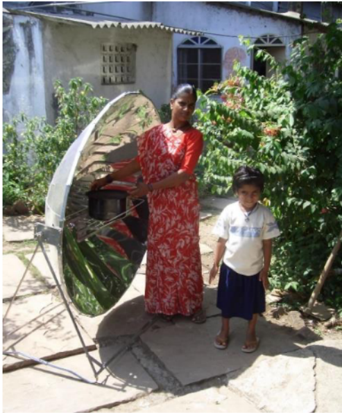
Photo E9: Operating the pot in the shadow of the reflector
