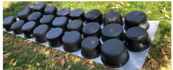
The aluminium pots are spray-painted with fireproof paint.
