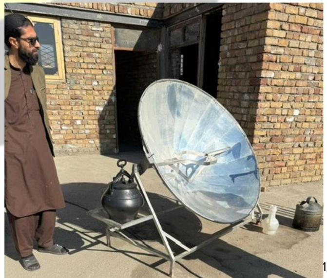
On site, 100 ready-to-use solar cookers were built and assembled in a suitably equipped workshop and thereafter distributed to 100 user families – partly locally in Khost, partly in villages in the Khost province.
